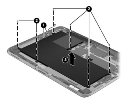
Reverse this procedure to install the battery.
